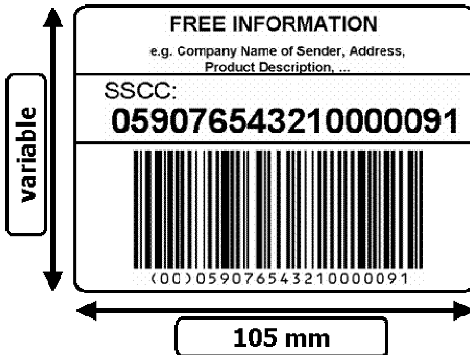
Figure 3. GS1 Logistic Label with SSCC only.
